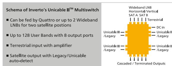
The existing legacy multiswitch can be replaced with an Inverto future-proof Unicable II® Multiswitch, allowing to connect multiple receivers at the home over a single coax cable with unlimited access to all the satellite services.
