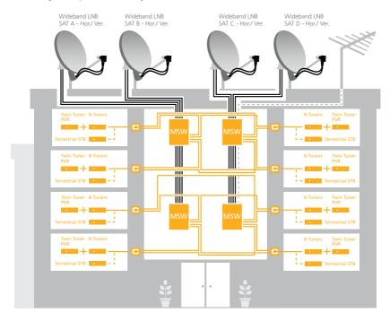
Connect the cables from the Quattro/Wideband LNB to the input connectors (pay attention to identification of the connectors and the correct position of the LNB type switch) and connect the Terrestrial antenna to Terrestrial input port:
