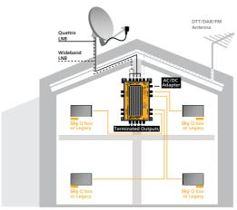
The following diagram illustrates a typical MDU/building installation with two Wideband LNBs receiving two satellites:
